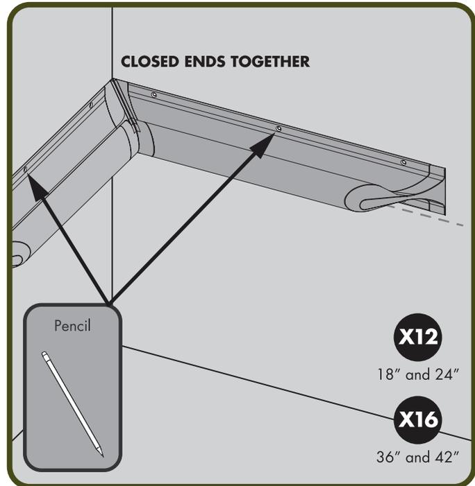
2 Check to make sure there are minimal gaps between two Grab Bars and between Grab Bars to the wall. Use the appropriate drill bit to drill the appropriate number of holes on the previously marked location.
