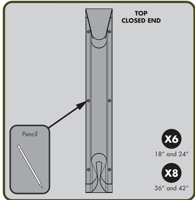
2 Use the appropriate drill bit to drill the appropriate number of holes on the previously marked location.
