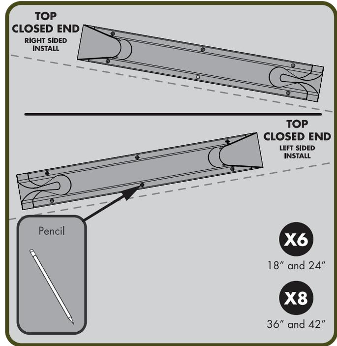
3 Use the appropriate drill bit to drill the appropriate number of holes on the previously marked location.
